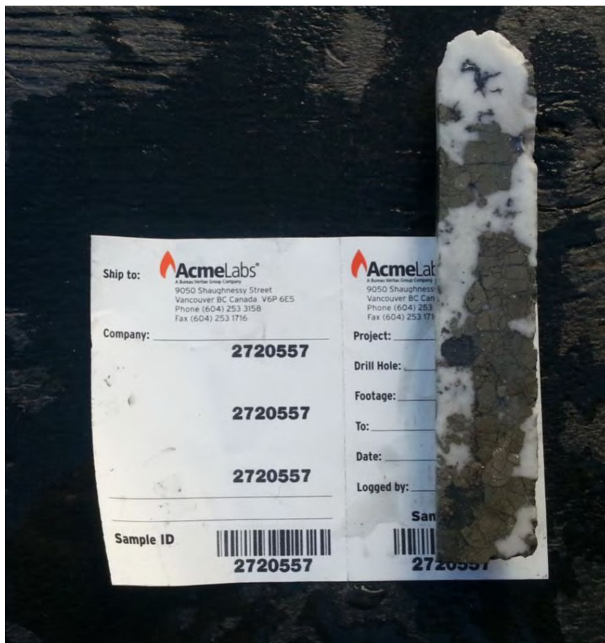
FIGURE 10.6 PHOTOGRAPH OF SIF CARBON DRILL CORE TETRAHEDRITE AND PYRITE MINERALIZATION
